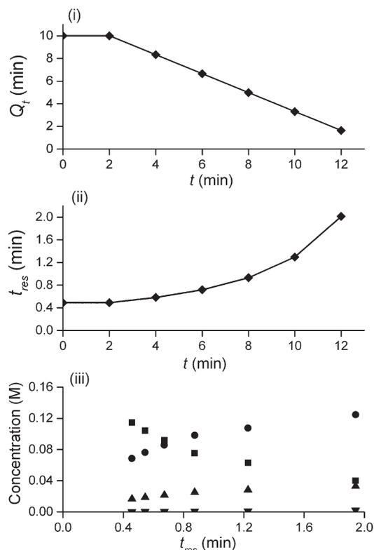
Fig. 3 i) Total volumetric flow rate ( $Q_{total}$ ) change throughout the duration of a ramp,  $\diamond$  HPLC injection; (ii) residence time,  $\tau$ , as a function of operation time,  $t$ ; (iii) resulting concentration-residence time profile generated from a typical multi-step reaction scenario,  $\blacksquare$  2,4-DF 1,  $\bullet$  *ortho*-3,  $\bullet$  *para*-4,  $\blacktriangledown$  *bis*-5.
