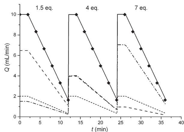
**Fig. 2** Changes in volumetric flow rate over time, where  $Q_{P1}$ ,  $Q_{P2}$ ,  $Q_{P3}$  and  $Q_{\text{total}}$  were for ..... pump 1 (Ar in EtOH), --- pump 2 (EtOH), -.- pump 3 (pyrrolidine in EtOH), — total volumetric flow rate, and ♦ HPLC injection points respectively. The linear flow ramps correspond to pyrrolidine 2 to 2,4-difluoronitrobenzene 1 molar ratios: (i) 1.5 : 1 and (iii) 7 : 1 using  $Q_{\text{total}}$  from 10 to  $1.5 \text{ mL min}^{-1}$ .
