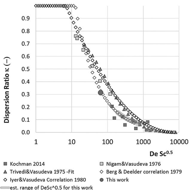
Fig. 4 The dispersion ratio  $\kappa$  vs.  $De Sc^{0.5}$  for various literature data. Where possible data have or correlations have been taken from the papers. If the data could not be retrieved and no correlation was given the data has been fitted with a line that visually represents the data well.
