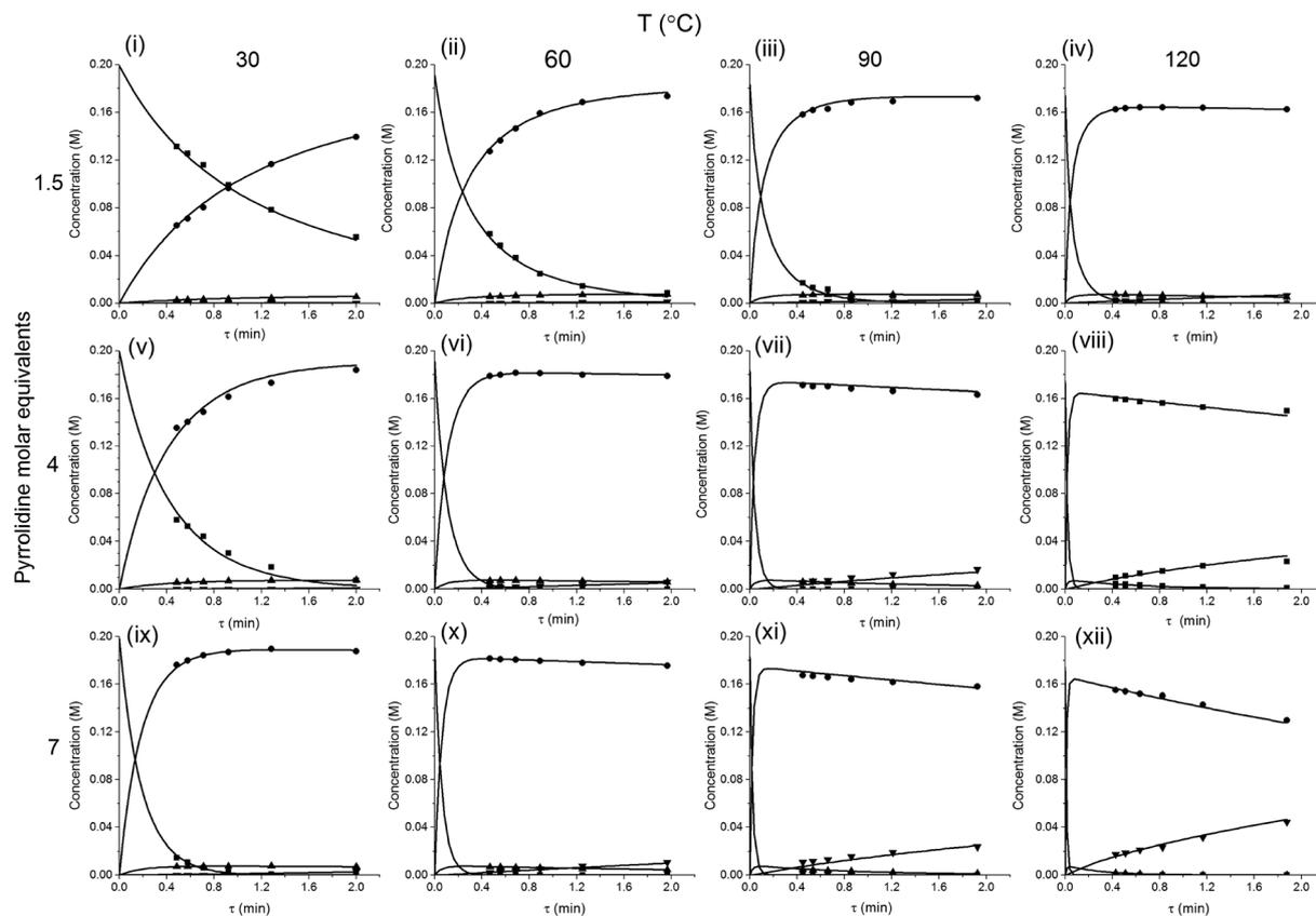
Fig. 5 Concentration-time profiles from simultaneous parameter fitting, points = experiments ■ 2,4-DF 1, ● *ortho*-3, ● *para*-4, ▼ bis-5, lines = model using Table 1 kinetic parameter estimates (i–xii).
