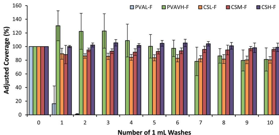
Fig. 3 Lab-scale wash-off profiles for 5 fluorescently labeled polymers. Droplets of polymer formulations were allowed to dry on leaves and imaged prior to sequential washing and re-imaging. Image analysis was used to quantify coverage and by adjusting the coverage value of dry deposits to represent 100% coverage. Results are presented as mean values ( $n = 3$ )  $\pm$  standard deviation.
