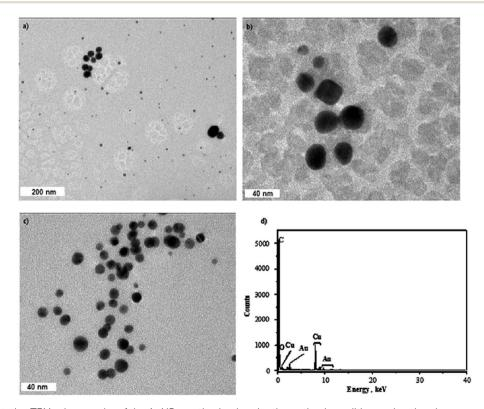
Fig. 5 The representative TEM micrographs of the AuNPs synthesized under the optimal conditions using the plasma-reaction system with the FLA (a–c) along with the EDXMA spectra (d).
