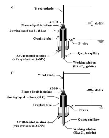
Fig. 1 The plasma-reaction systems based on the APGD sustained in the surrounding air between the solid pin electrode and the FLA (a) or the FLC (b).
