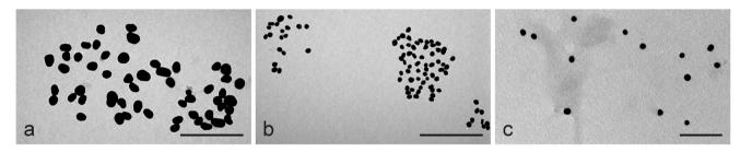
Fig. 2 AuNPs in TEM images. (a) Oval-shaped 80 nm AuNPs. (b) Spherical 40 nm AuNPs. (c) Spherical 15 nm AuNPs. Scale bars are 500 nm in (a) and (b) and 100 nm in (c).
