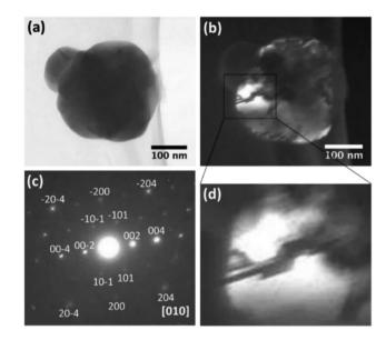
Fig. 5 TEM images of CZTS nanocrystals in bright (a) and dark field (b) taken in the superlattice reflection g = 002 illustrated by the selected area electron diffraction pattern (c). Expanded dark field image highlighting contrast arising from ADBs (d).
