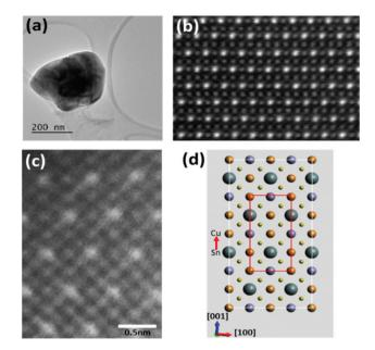
TEM image of the entire CZTS nanocrystal (a). Atomic resolution high angle annular dark field (HAADF) images (b-c). (d) Schematic representation of an expanded unit cell describing all atomic columns of elements (Cu, Zn, Sn and S) visible in (c).
