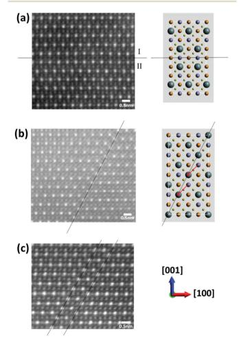
Fig. 3 Atomic resolution HAADF images of antisite domain boundaries (ADBs) showing fault displacement of  $\frac{1}{2}[110]$  (a),  $-\frac{1}{4}[201]$  (b) and  $-\frac{1}{2}[201]$  (c).
