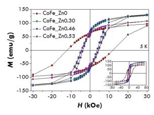
Fig. 3 Magnetisation *versus* magnetic field curves at 5 K of the  $CoFe_Z nx$  (with x = 0, 0.30, 0.46, 0.53) samples.
