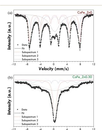
Fig. 7 Room temperature Mössbauer spectra of the samples CoFe\_Zn0 (a) and CoFe\_Zn0.30 (b).
