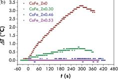
**Fig. 6** (a) Magnetisation *versus* magnetic field curves of CoFe\_Znx (with x = 0, 0.30, 0.46, 0.53) samples measured at 300 K. (b) Heating curves of CoFe\_Znx (with x = 0, 0.30, 0.46, 0.53) samples at 25 °C, obtained under a magnetic field of 183 kHz and 17 kA m<sup>-1</sup>.
