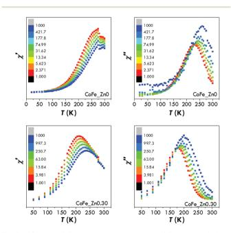
Fig. 8 AC susceptibility measurements. In phase  $(\chi')$  and out of phase  $(\chi'')$  components measured at 1, 4, 16, 63, 251 and 997 Hz as a function of the temperature for samples CoFe\_Zn0 (upper panels) and CoFe\_Zn0.30 (bottom panels).
