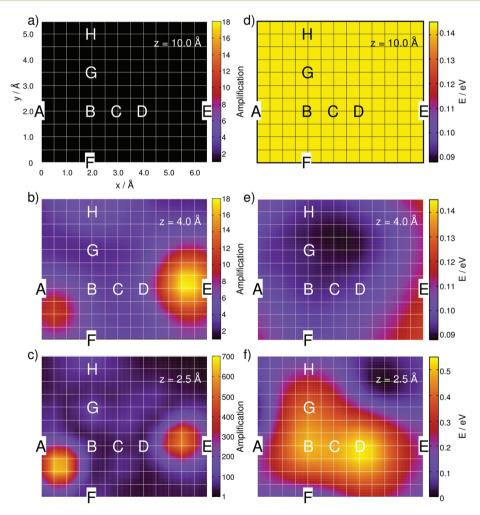
Fig. 2 Simulated integrated Raman signal amplification based on eqn (3) along the grid at (a) z = 10 Å, (b) 4 Å and (c) 2.5 Å for the one-silver-atom model. (d)–(f) illustrate the relative ground state potential energy surfaces (*E* in eV) of the respective layers. Notice the adjusted color bars scales for the amplification and energy in (c) and (f).
