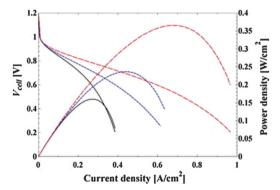
**Fig. 9** PEMFC performance when fractal distributors are used as bipolar plates: (black line – 16 branches; blue line – 64 branches and black line – 256 branches). <sup>98</sup> Reprinted from ref. 98 with permission from Elsevier.
