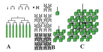
Fig. 6 (A) Set of 1D distributors feeding progressively larger 1D arrays (vectors); (B and C) extension of the scalable, fractal distributor concept to 2D and 3D, respectively. 47 Copyright 2015 Wiley.
