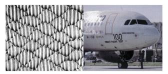
The riblets on shark skin (left) provided the inspiration for the creation of a plastic film with the same microscopic texture used as coating for the airplane wings (right).<sup>27</sup> Copyright 1999, Rights Managed by Nature Publishing Group.
