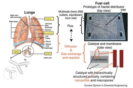
Fig. 7 Fuel cell design guided by the architecture of the lung and the associated physical mechanisms.<sup>47</sup> Copyright 2015 Wiley.
