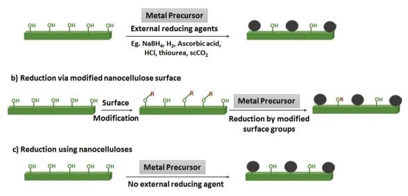
Fig. 2 Three approaches for synthesis of metal NP-nanocellulose hybrid composite: (a) reduction using an external agent, (b) reduction via modified nanocellulose surface, and (c) reduction using nanocelluloses.
