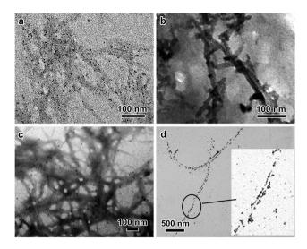
Fig. 3 TEM images of metal NPs supported by CNCs: (a) Pd on wood pulp CNCs (reproduced from Cirtiu et al.3 by permission of The Royal Society of Chemistry); (b) Pt on cotton CNCs (reproduced from Benaissi et al.5 by permission of The Royal Society of Chemistry); (c) Au on wood pulp CNCs (reproduced from Lam et al.9 by permission of The Royal Society of Chemistry); (d) Cu on tunicate CNCs (reprinted with permission from Padalkar et al. 13 Copyright 2010 American Chemical Society).
