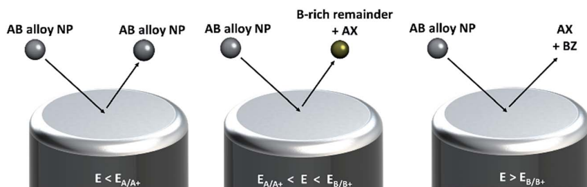
Fig. 1 Schematic drawing of nano impact experiments of bimetallic alloy nanoparticles.
