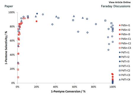
Fig. 6 Summary of 1-pentyne hydrogenation performance for PdSn and PdTi catalysts. Note that the data arises from experiments performed at a range of temperatures from room temperature to  $250\,^{\circ}$ C.
