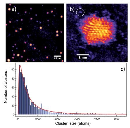
Fig. 10 (a) HAADF STEM image of Ag clusters created in the MACS. (b) A high-resolution image of one such Aq cluster, the circled region shows a single Aq atom, as used for mass calibration. (c) Size distribution of the clusters produced, calculated from the integrated HAADF STEM intensities.
