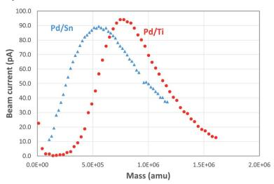
Fig. 2 Mass spectra of Pd/Sn and Pd/Ti clusters. The clusters' size distribution varies with magnetron sputtering conditions, two examples are shown here. It's estimated that both types of clusters shown in this figure have a diameter around 5 nm.
