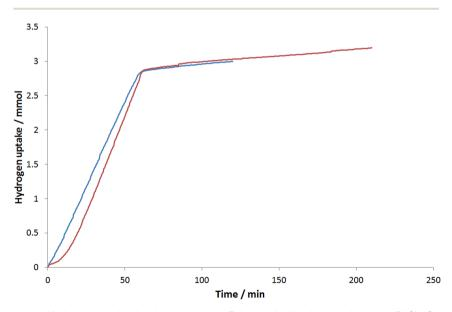
Fig. 7 Hydrogen uptake data in the selective 3-hexyn-1-ol hydrogenation using  $Pd/Al_2O_3$  (blue) and  $PdTi/Al_2O_3$  (red) catalysts prepared *via* the clusterbeam technique. The steeper slope between 0 and 60 minutes is the hydrogenation of 3-hexyn-1-ol (R1), whilst the shallower slope above 60 minutes is the hydrogenation of *cis*- and *trans*-3-hexen-1-ol (R3 + R4).
