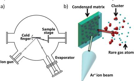
Fig. 9 (a) Scheme of the Matrix Assembly Cluster Source (MACS) employed in the work, showing the ion gun (Omicron ISE-5), the cryogenically cooled matrix, the sample collection stage and the evaporator (Createc effusion cell). (b) Schematic of the MACS process.
