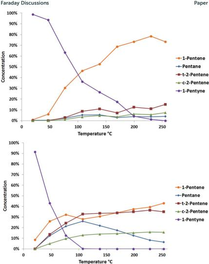
Fig. 5 Data for the catalytic 1-pentyne hydrogenation with PdTi/ $\gamma$ -Al<sub>2</sub>O<sub>3</sub> (top) and Pd/ $\gamma$ -Al<sub>2</sub>O<sub>3</sub> (bottom) prepared using the clusterbeam method. The charts show the outlet concentration of each compound at different reaction temperatures.
