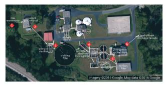
Fig. 2 Aerial view of Northfield WWTP with six sampling locations for the liquid stream: 1) raw wastewater, 2) preliminary effluent, 3) primary effluent, 4) secondary trickling filter, 5) secondary activated sludge system, and 6) final effluent.
