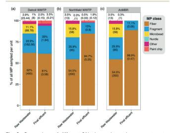
**Fig. 6** Comparison of different SAL shape classes in raw wastewater *versus* final effluents at the three WWTPs. Percentage of each class of total SAL sampled per unit is depicted. Absolute number of SAL per liter (or average, where replicates exist) is noted in parentheses.
