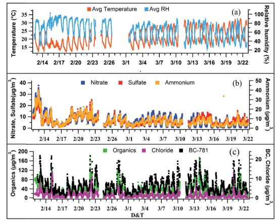
Fig. 1 (a) Time series (15 min resolution) of temperature (T, °C) and relative humidity (RH, %). (b) Nitrate, sulfate and ammonium mass concentrations ( $\mu$ g m<sup>-3</sup>). (c) Organics, chloride, and BC concentrations ( $\mu$ g m<sup>-3</sup>).
