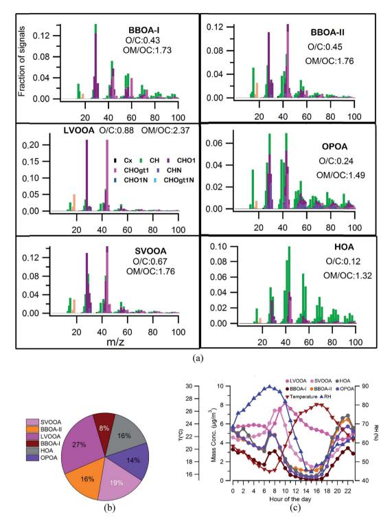
Fig. 4 AMS-PMF factors for OAs: (a) the m/z spectra for the 6 factor solution, (b) percent contribution of the different factors resolved in PMF, and (c) the diurnal profiles of the different OA factors and meteorological parameters (RH & T).
