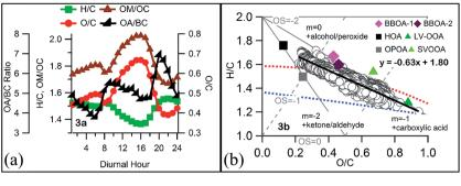
Fig. 3 (a) Diurnal variations of elemental and OA/BC ratios (b) Van Krevelen diagram showing the evolution of organic aerosols along with H/C and O/C of the identified OA factors from this study
