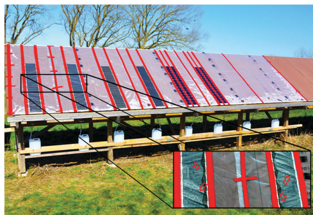
Fig. 1 Rain run-off leaching setup at DTU, Risø campus (Denmark), used to study the emission of elements to the environment from organic solar cells during operation and failure. At the end of each row, a gutter collects the rain (and fog/dew), and a plastic tube guides this to a storage canister. The inset shows the damage caused deliberately in some Ag-OPV samples (see text for further details).
