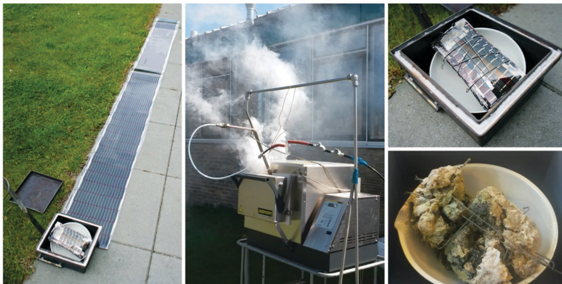
Fig. 1 Left: Picture of 1 m 2 of an organic solar cell rolled out on the ground. On the bottom left of the same picture an additional 1 m 2 has been cut into smaller pieces, tied up with heat resistant steel wire and put in a ceramic bowl inside the steel container. Middle: Picture of the oven setup with the steel container placed inside the high temperature oven with a controlled air flow. Right: Pictures of the cut up solar cells before and after incineration.
