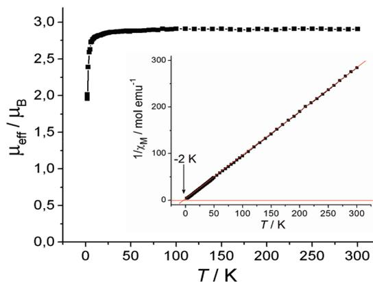
**Fig. 2** Temperature dependence of the effective magnetic moment of **1** in the 1.9–300 K range. The inset shows the temperature dependence of the reciprocal molar magnetic susceptibility of **1** in the same range.
