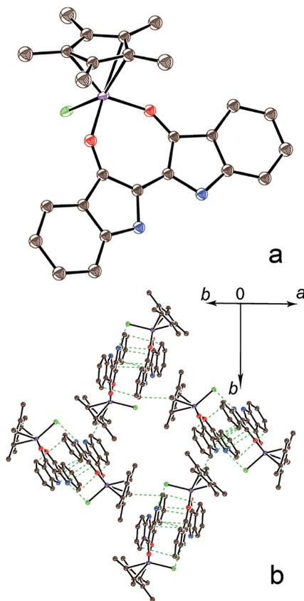
**Fig. 1** (a) Molecular structure of the coordination complex (oxygen atoms are red, nitrogen atoms are blue, chloride anions are green, and chromium atoms are violet). Hydrogen atoms are not shown. (b) van der Waals contacts between the components are shown by green dashed lines.
