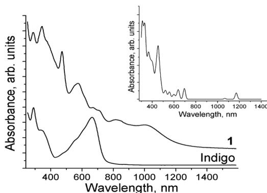
**Fig. 5** Spectrum of indigo and **1** in the UV–visible–NIR range recorded in KBr pellets. The pellet for **1** was prepared under anaerobic conditions. The inset shows the theoretical spectrum calculated for the optimized structure of **1**.
