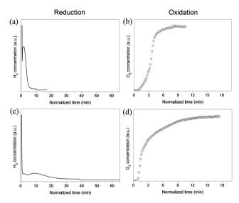
Fig. 3 Redox reactions of 1.9 wt% Ni-doped Pr<sub>2</sub>O<sub>2</sub>SO<sub>4</sub> at 700 °C (a, b) and 600 °C (c, d) under feed stream of 10% H<sub>2</sub>/Ar and 5% O<sub>2</sub>/He.
