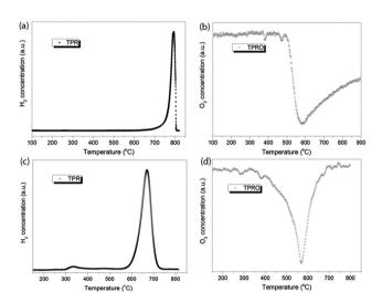
Fig. 2 Temperature programmed profiles of redox reactions catalyzed by nanoparticulate Pr<sub>2</sub>O<sub>2</sub>SO<sub>4</sub>: on the left are TPR profiles of non-doped (a) and 1.9% Ni-doped (c) Pr<sub>2</sub>O<sub>2</sub>SO<sub>4</sub> in a flow of 10% H<sub>2</sub>/Ar and on the right are TPRO profiles of non-doped (b) and 1.9% Ni-doped (d) Pr<sub>2</sub>O<sub>2</sub>SO<sub>4</sub> in a flow of 20% O<sub>2</sub>/He. Heating rate 10 °C min<sup>-1</sup>.
