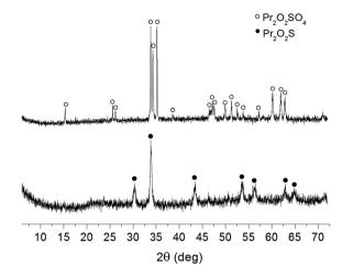
Fig. 1 Powder XRD patterns of nanoparticulate Pr<sub>2</sub>O<sub>2</sub>SO<sub>4</sub> obtained by miniemulsion method, and Pr<sub>2</sub>O<sub>2</sub>S, resulted from the subsequent reduction.
