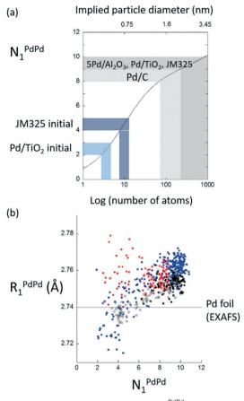
Fig. 7 (a) Shows the relationship between  $N_1^{\rm PdPd}$  and the average fcc Pd particle size of the initial (blue) and final (grey) states of the catalysts; Fig. 7 (b) the correlations obtained between  $R_1^{\rm PdPd}$  and  $N_1^{\text{PdPd}}$  along with the average value of  $R_1^{\text{PdPd}}$  returned from analysis of the reference foil: black solid circles = Pd/Al<sub>2</sub>O<sub>3</sub>; black open circles =  $Pd/Al_2O_3$  (JM325); red = Pd/C; blue = Pd/TiO<sub>2</sub>.
