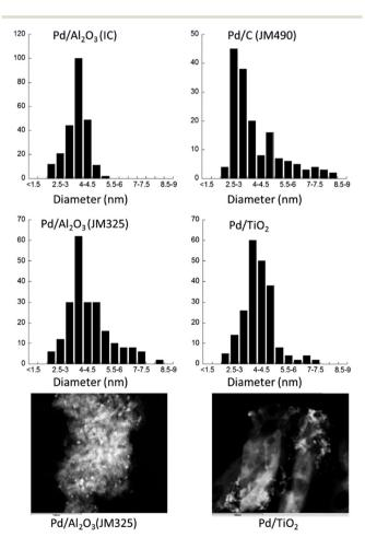
Fig. 1 Particle size distributions obtained by TEM for each of the four supported Pd catalysts (all 5 wt% loading). Representative images for the Pd/Al<sub>2</sub>O<sub>3</sub> (JM325) and Pd/TiO<sub>2</sub> samples are also given.
