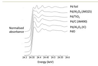
Fig. 2 Normalised Pd K-edge XAFS for four different 5 wt% Pd catalysts in their native "dry" states. Spectra from a bulk PdO and a Pd foil are also given.
