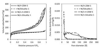
Fig. 2 N2-Physisorption isotherms and pore size distributions of Ni catalysts
