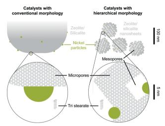
Fig. 6 Graphical representation of catalysts with conventional and nano-structured morphology.
