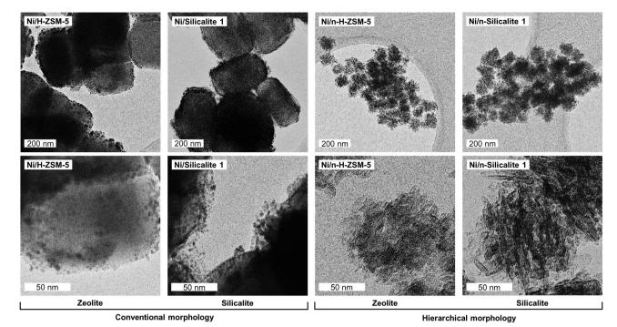
Fig. 1 Representative micrographs of Ni supported on (n)-H-ZSM-5 and (n)-Silicalite 1 materials. Note the cross-linking between crystalline sheets for the nanosheet materials (n-H-ZSM-5 and n-Silicalite 1), which produces mesoporosity. The dark dots in all images are nickel particles.
