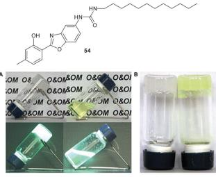
Fig. 34 Chemical structure of gelator 51 and photographs of CCl<sub>4</sub>-gel of 51 (1% (w/v)) (A) before (left) and after (right) adding DCP liquid (100 equiv.) under ambient (top) and UV (bottom) light and (B) before (left) and after (right) exposure to DCP vapour. Figure adapted from ref. 100 with
