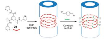
**Fig. 19** Self-assembling compound **29** and its covalent capture through surface crosslinking with 1,4-bis(bromomethyl)benzene. Figure adapted from ref. 69 with permission.
