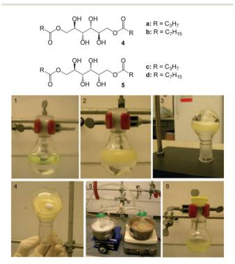
Fig. 5 Chemical structures of sugar-based gelators 4 and 5 and images 1-6 showing the immobilisation of bulk diesel from its two-component mixtures with water, and recovery of the oil by distillation. Figure adapted from ref. 25 with permission
