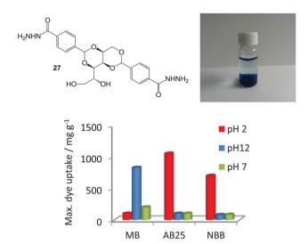
Fig. 17 Chemical structure of DBS acylhydrazide (DBS-CONHNH<sub>2</sub>, 27), photograph of gel extracting methylene blue from basic water and the maximum dye adsorption onto 27 supramolecular gel under various conditions of pH. Figure adapted from ref. 58 with permission.
