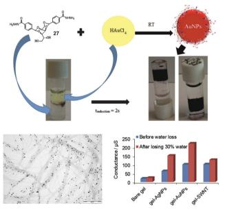
Fig. 24 Scheme showing uptake of noble metal and in situ reduction to nanoparticles by hydrogel nanofibres of DBS-CONHNH<sub>2</sub> (27), TEM image showing nanoparticles aligned along gel nanofibres and enhanced conductances of the nanoparticle-embedded gels compared with bare gel, and gels containing single walled nanotubes. Figure adapted from ref. 80
