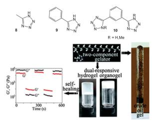
Fig. 8 (top) Chemical structures of 8, 9, and 10; (bottom left) a loop test of hydrogel of L-octylamine via continuous step-stress measurement at 1 Hz: (bottom right) photos of dual responsive gels and inverted crude oil gel. Figure adapted from ref. 29 with permission.
