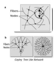
Fig. 38 Illustration of fibre networks commonly observed in supramolecular materials. (a) Interconnecting fibre network consisting of fibres and joints (or nodes) with closed loops. (b) Cayley tree-like network (left) with open loops, and spherulites. Figure adapted from ref. 113 with permission.
