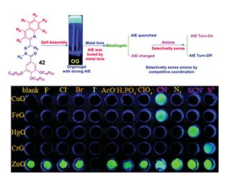
Fig. 28 Gelator 42 self-assembles and has its assembly induced emission (AIE) tuned by the presence of metal ions. The emission of different metallogels is then tuned by the presence of certain anions, allowing the sensor to detect CN<sup>-</sup>, SCN<sup>-</sup> and S<sup>2-</sup> via an 'array mode' of sensing. Figure reproduced from ref. 92 with permission.
