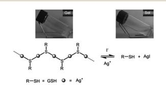
Fig. 26 Illustration of reversible gel-sol state transition of supramolecular hydrogel of Ag(i)-GSH coordination polymers (where R-SH is glutathione, GSH) triggered by alternately adding I<sup>-</sup> into the hydrogel, or additional Ag(I) into the resulting sol. Figure reproduced from ref. 89 with permission.
