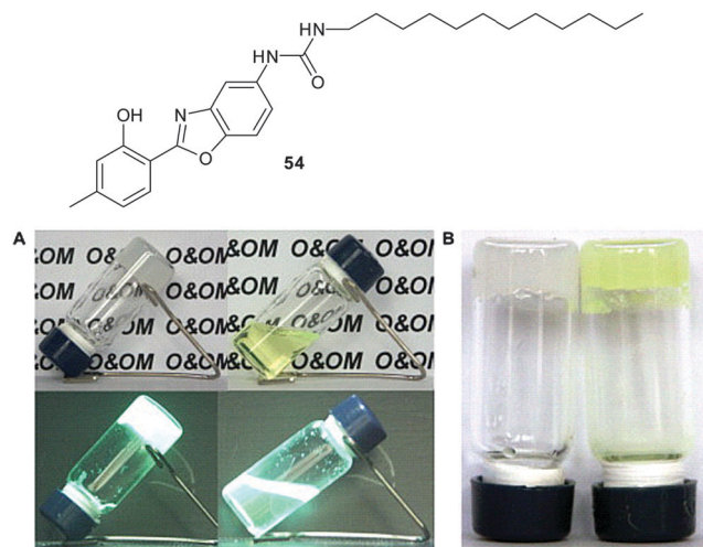
Fig. 34 Chemical structure of gelator 51 and photographs of \text{CCl}_4 -gel of 51 (1% (w/v)) (A) before (left) and after (right) adding DCP liquid (100 equiv.) under ambient (top) and UV (bottom) light and (B) before (left) and after (right) exposure to DCP vapour. Figure adapted from ref. 100 with permission.
