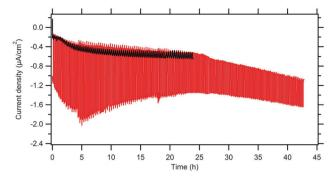
Fig. 5 Long-term chronoamperometric measurement of the diamond electrode sensitized with **P1** (red curve) and the blank, non-sensitized diamond electrode (black curve). Chopped white light illumination (100 mW cm $^{-2}$ ; simulated AM 1.5G solar spectrum, 10 min dark/light interval). Electrolyte solution: 5 mM dimethylviologen in 0.1 M Na<sub>2</sub>SO<sub>4</sub>, pH 7. Applied potential bias: -0.3 V vs. Ag/AgCl.
