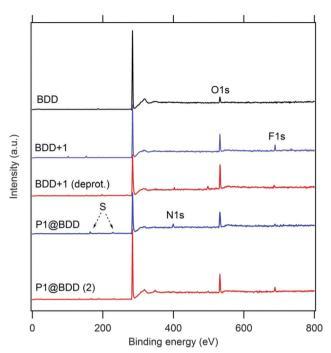
Fig. 3 XPS spectra of the studied samples. **P1@BDD** is the optimized sample with linker **1**; **P1@BDD** (2) is another sample with linker **2**. Curves are offset for clarity, but the intensity scale is identical for all spectra.
