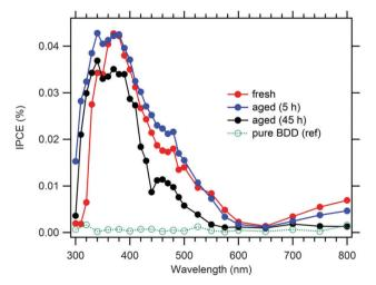
Fig. 6 IPCE spectrum for the fresh **P1@BDD** electrode and that after passing 4 or 45 hours of photoelectrochemical test with chopped illumination at 1 Sun (aged). A reference spectrum for pristine, non-sensitized BDD electrode is also shown. Electrolyte solution 0.1 M  $Na_2SO_4 + 5$  mM dimethylviologen; bias voltage -0.3 V vs. Ag/AgCl.
