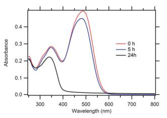
Fig. 7 UV-Vis spectrum of the solution of the **P1** dye in absolute ethanol (starting concentration  $10^{-5}$  mol L<sup>-1</sup>). Optical length 1 cm. The spectrum of a fresh solution (red curve) and that after illumination with a white light of 1 Sun intensity for 5 hours (blue curve) or 24 hours (black curve).
