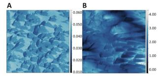
Fig. 3 SNIM images:  $5\times 5~\mu m$  of the Au electrode surface. Mechanical amplitude signal (A) and optical signal (B).
