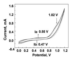
**Fig. 2** Cyclic voltammogram of a Tröger's base derivative **6** in CH $_3$ CN/TBAFB/HCl on a Pt electrode. The electrode potential was swept repeatedly between 0.0 and 1.2 V vs. Ag/AgCl at a scan rate of 50 mV s $^{-1}$ ; the number of scans is 4. $\dot{\uparrow}$
