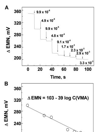
Fig. 5 (A) Potentiometric response and (B) calibration graph of the electrode modified with the polymer based on  $\bf 6$  towards VMA in 0.1 mol L<sup>-1</sup> phosphate buffer at pH = 7.
