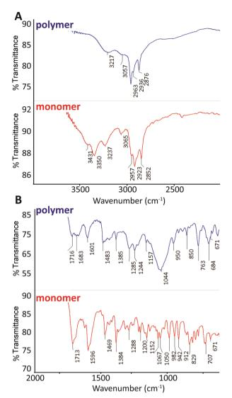
Fig. 4 FTIR spectra of the polymer (blue) and the monomer (red) from 4000 to 2000  ${\rm cm^{-1}}$  (A) and from 1900 to 600  ${\rm cm^{-1}}$  (B). Each spectrum was averaged from 256 scans with 4  ${\rm cm^{-1}}$  resolution.
