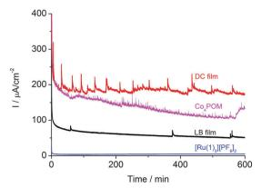
Fig. 3 Current densities of LB and DC films, and DC  $Co_4POM$  and  $[Ru(\mathbf{1})_3][PF_6]_2$  films during chronoamperometry (+1.3 V bias vs. Ag/AgCl). Spikes are caused by surface bubble formation.
