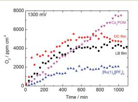
Fig. 2  $O_2$  evolution vs. time at +1.3 V bias for LB and DC films prepared from  $[Ru(\mathbf{1})_3][PF_6]_2$  and  $Co_4POM$ , and separate DC  $Co_4POM$  and  $[Ru(\mathbf{1})_3][PF_6]_2$  films.
