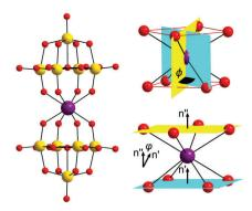
Fig. 1 Molecular structure (left) and representations of the two distortion angles of the Tb coordination (right) for the [Tb(W<sub>5</sub>O<sub>18</sub>)<sub>2</sub>]<sup>9-</sup> polyanion in **Tb**; atom colour code: W (yellow), O (red) and Tb (violet).
