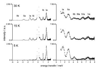
Fig. 2 Variable temperature INS spectra of  $\mathbf{Tb^D}$ . Left:  $\lambda = 4.74 \, \text{Å}$ , integration interval 0.8 Å $^{-1}$  < Q < 1.2 Å $^{-1}$  and right:  $\lambda$  = 2.37 Å, integration interval 1.15  $\mbox{Å}^{-1} < Q <$  1.65  $\mbox{Å}^{-1}$ . Positive numbers correspond to neutron energy loss.
