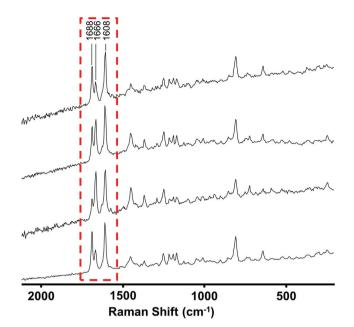
Fig. 3 Raman spectra recorded at 4 different positions in a mixed sample showing point-to-point variation in relative signal intensities. Spectra are vertically offset for clarity.
