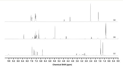
Fig. 7 <sup>1</sup>H-NMR Spectra of (a) 4-methylbenzylcathinone (b) AB-FUBINACA (c) 5-EAPB. Spectra are vertically offset for clarity.
