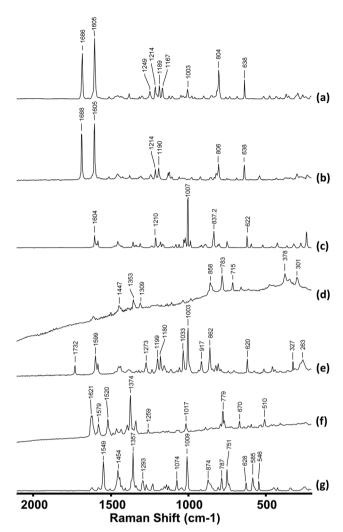
Fig. 2 Raman spectra of (a) mephedrone, 4-MMC (b) 4-methylethcathinone, 4-MEC (c) methamphetamine (d) 5,6-MDAI (e) ethylphenidate (f) AM-2201 (g) N,N-dimethyltryptamine. Spectra are vertically offset for clarity.
