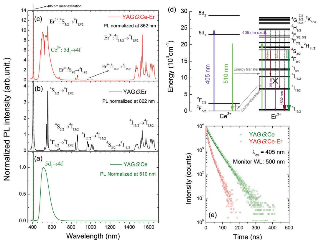
Fig. 1 PL spectra of the (a) YAGG:Ce, (b) YAGG:Er and (c) YAGG:Ce–Er ceramic samples under 405 nm laser excitation; (d) energy level diagrams of Ce<sup>3+</sup> and Er<sup>3+</sup>; (e) fluorescence decay curves of the YAGG:Ce and YAGG:Ce–Er ceramic samples ( $\lambda_{\text{ex}} = 405$  nm and  $\lambda_{\text{em}} = 500$  nm).
