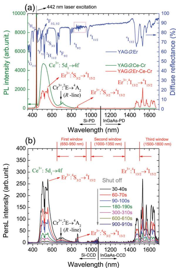
Fig. 2 (a) PL spectra of the YAGG:Ce–Cr and YAGG:Er–Ce–Cr ceramic samples ( $\lambda_{ex} = 442$  nm) as well as the diffuse reflectance of the YAGG:Er ceramic sample (pink-dotted-line area is the detector change region from PMT to PbS). (b) PersL spectra of the YAGG:Er–Ce–Cr ceramic sample (integrating time: 10 s) after ceasing the blue light illumination.
