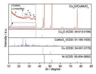
Fig. 2 XRD patterns of the as-synthesized electrode.
