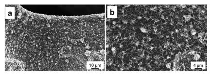
Fig. 6 SEM images of the Cu<sub>2</sub>O/CuMoO<sub>4</sub> nanosheet electrode after charge-discharge for 3000 cycles at a current density of 5 A g<sup>-1</sup>.
