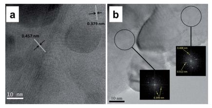
Fig. 3 (a and b) TEM images of Cu<sub>2</sub>O/CuMoO<sub>4</sub> nanosheets and the corresponding Fourier transform patterns (inset of b).
