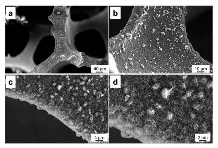
Fig. 1 Typical SEM images of Cu<sub>2</sub>O/CuMoO<sub>4</sub> nanosheets on Ni foam at different magnifications
