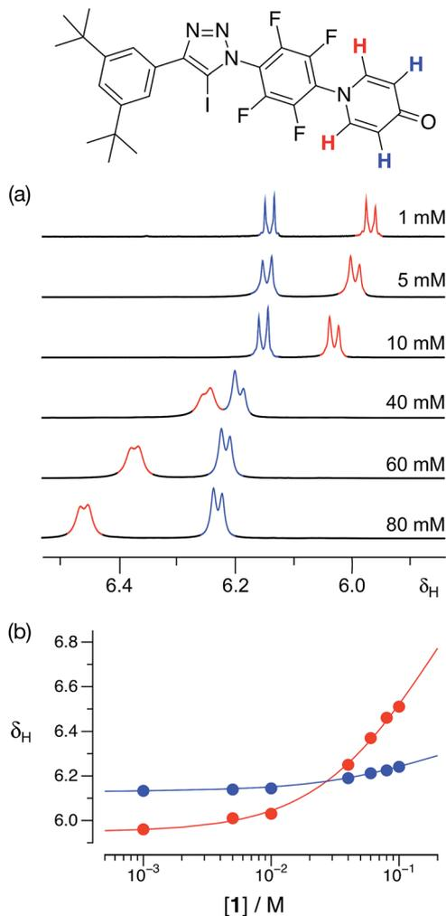
Fig. 4 (a) Partial 500.1 MHz  $^1\text{H}(^{19}\text{F})$  NMR spectra of iodotriazole **1** at various concentrations in  $d_8$ -toluene at 293 K showing the  $^1\text{H}$  resonances arising from the pyridone ring protons. (b) Best fits (solid lines) of the changes in the chemical shifts of the  $^1\text{H}$  resonances arising from the pyridone ring protons as a function of concentration to a  $1 + 1 \rightleftharpoons [1 \cdot 1]$  dimerisation model.
