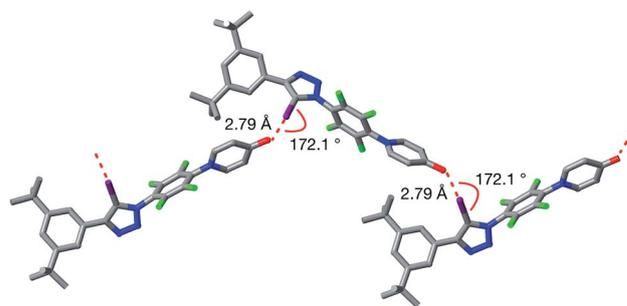
Fig. 3 Solid state structure of **1** determined from single crystal X-ray diffraction data. Halogen bonds are marked as red dashed lines ( $r(\text{O}\cdots\text{I}) = 2.790 \text{ \AA}$ ;  $\angle(\text{O}\cdots\text{I}-\text{C}) = 172.1^\circ$ ). Atom colouring: C atoms = grey, N atoms = blue, O atoms = red, I atoms = purple. Hydrogen atoms and included solvent of crystallisation (toluene) are omitted for clarity.
