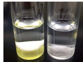
Fig. 9 Dichloromethane solutions of phosphino-stiborane 7 layered with water (left) and 0.1% aqueous formaldehyde (right) after sonication for 90 min.
