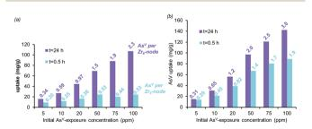
Fig. 4 The  $As^{V}$ -adsorption isotherms for AcOH-UiO-66 $|_{11/12}$  (a) and  $HCl-UiO-66|_{9/12}$  (b) at short (0.5 h) and long (24 h) exposure time, plotted as bar graphs with the  $\mbox{As}^{\mbox{\scriptsize V}}$  :  $\mbox{Zr}_{\mbox{\scriptsize 6}}$  ratios indicated at the top of each bar. Experimental conditions: batch exposure of a sample of MOF (10 mg) to the appropriate AsV-containing solution (30 mL).
