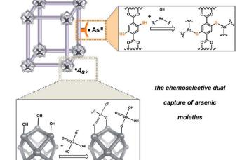
Fig. 1 A schematic representation that suggests how MOFs can be tailored to coordinate anionic As<sup>V</sup> moieties at the node while binding neutral As<sup>III</sup> with the linkers.
