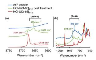
Fig. 5 DRIFTS spectra of HCl-UiO-66 $|_{9/12}$  sample before and after As<sup>V</sup> treatment, showing the presence of -As-O-H bonds after exposure. Spectra for powder Na<sub>2</sub>HAsO<sub>4</sub>·7H<sub>2</sub>O are included as reference. Data for AcOH-UiO-66 $|_{11/12}$  can be found in the ESI,† Fig. S14.
