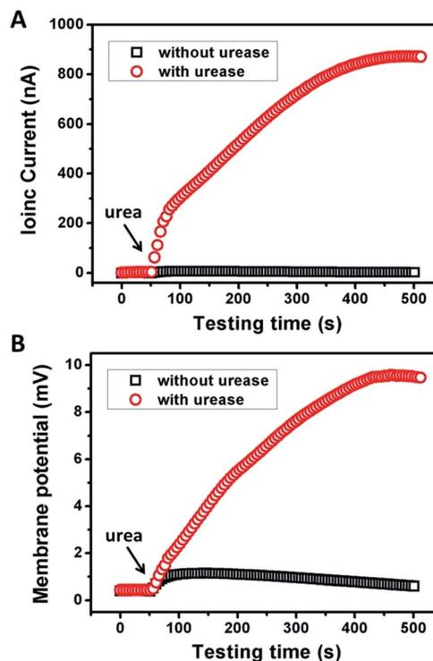
Fig. 2 Response of (A) ionic current and (B) membrane potential of GPM under urea triggered enzymatic catalysis. Electrolyte: 0.01 mM KCl, pH 7. The concentrations of urease and urea were 0.5  $\text{mg mL}^{-1}$  and 10 mM, respectively.
