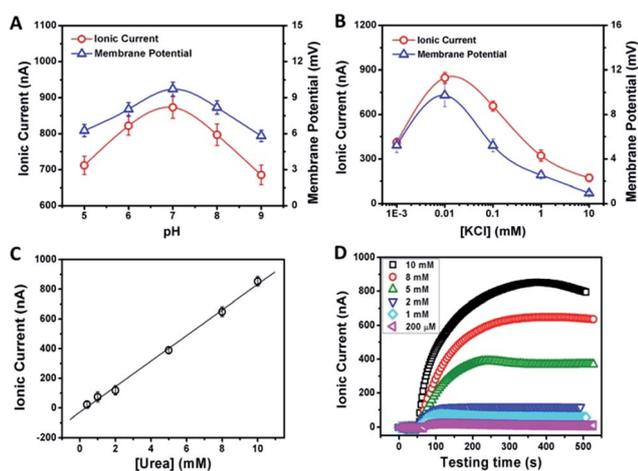
Fig. 3 pH (A) and concentration-dependence (B) of the ionic current and membrane potential generated from the urea-driven nanofluidic system. The concentrations of urease and urea were  $0.5 \text{ mg mL}^{-1}$  and 10 mM, respectively. (C) The dependence of ionic current on urea concentration. (D) Time dependency of ionic currents with respect to the urea concentration (the concentration of urease was  $0.5 \text{ mg mL}^{-1}$ ).
