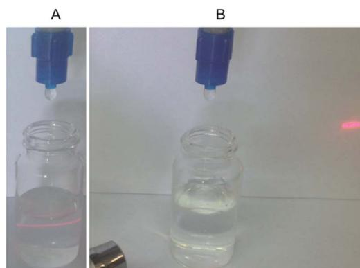
Fig. 9 (A) As-prepared **MOR-1**/sand column is washed with HCl acid (for protonation or regeneration of the sorbent) and then deionized water (to remove excess acid). As a result, **MOR-1** is coming through the column, since it forms a fine suspension as confirmed by the test with the laser beam. (B) The effluent collected after washing the **MOR-1-HA**/sand column with HCl acid and deionized water is a clear solution (as confirmed by the test with the laser beam).
