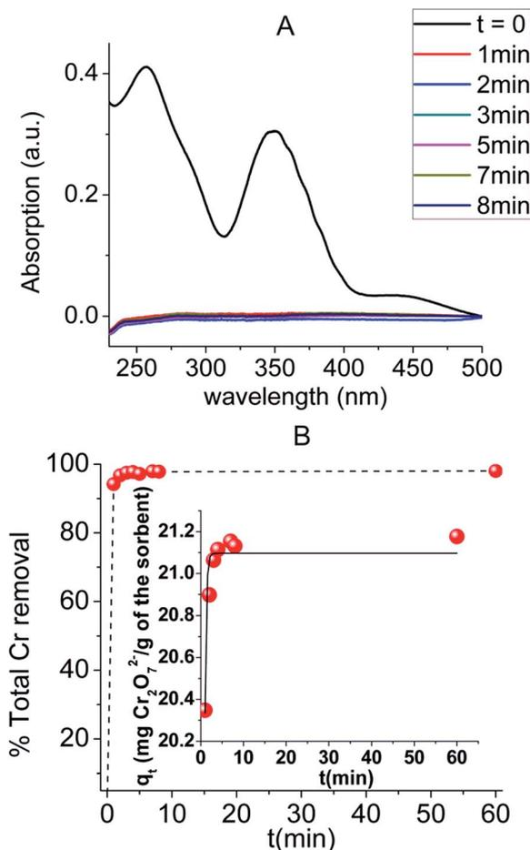
Fig. 6 (A) Selected UV-Vis data from the kinetic experiments (initial dichromate concentration = 21.6 ppm, pH  $\sim$  3). The  $\text{Cr}_2\text{O}_7^{2-}$  anions are not detectable after the sorption process with UV-Vis and thus, the dichromate concentrations of the solutions were determined by ICP-MS. (B) % Total Cr removal (determined by ICP-MS data) by MOR-1-HA vs. time (min). Inset graph: fitting of the kinetics data with the Lagergren's first-order equation.
