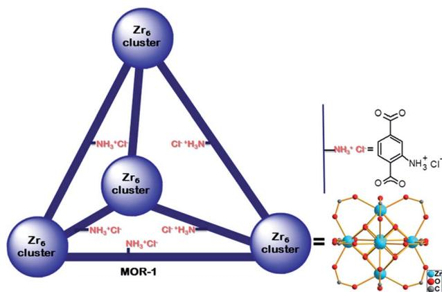
Fig. 1 Representation of the structure of (protonated) **MOR-1** material shown as a tetrahedral cage (based on the structure of UiO-66 material<sup>11</sup>).
