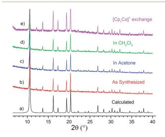
Fig. 1 Comparison of Powder X-ray Diffraction (PXRD) patterns of  $[TEA]_3[In_3(BTC)_4]$ : (a) calculated from the single crystal structure, (b) as synthesized, (c) after soaking for one day at 298 K in acetone or (d)  $CH_2Cl_2$  and (e) after  $[Cp_2Co]^+$  cation exchange in acetone.
