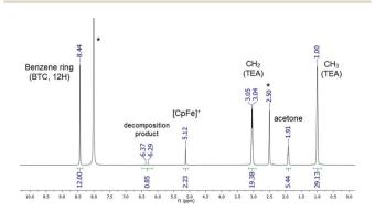
Fig. 7  $^{1}$ H NMR spectrum of [(Fp-L) $_{0.6}$ (TEA) $_{2.4}$ ][In $_{3}$ (BTC) $_{4}$ ] after digestion in DCl/d $^{6}$ -dmso (1/5 v/v). NMR solvent peaks are marked with an asterisk.
