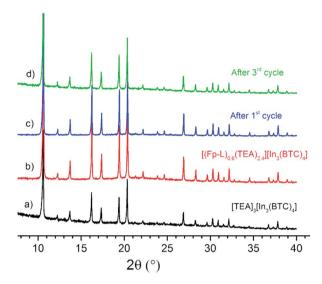
Fig. 6 Comparison of PXRD patterns between (a)  $[TEA]_3[In_3(BTC)_4]$  and  $[(Fp-L)_{0.6}(TEA)_{2.4}][In_3(BTC)_4]$  (b) as synthesized, (c) after one and (d) after three catalytic cycles.
