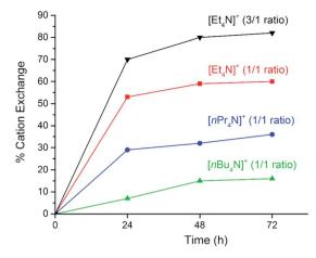
Fig. 2 Cation exchange (%) of [R<sub>4</sub>N]<sup>+</sup> by [Cp<sub>2</sub>Co]<sup>+</sup> determined by ICP-OES for  $[(Cp_2Co)_x(R_4N)_{3-x}][In_3(BTC)_4]$  (x = 3 corresponds to 100%). Conditions: 0.02 M solution of [Cp<sub>2</sub>Co][PF<sub>6</sub>] in acetone, initial ratio  $[R_4N]^+/[Cp_2Co]^+ = 1/1 \text{ or } 3/1$
