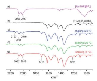
Fig. 5 Solid-state ATR IR spectra of (a)  $[Fp-THF][BF_4]$ , (b)  $[TEA]_3[In_3(BTC)_4]$  and  $[(Fp-L)_x(TEA)_3\__x][In_3(BTC)_4]$  prepared *via* cation exchange in acetone under different conditions: (c) shaking for 1 day at 25 °C, (d) soaking for 1 day at 25 °C and (e) soaking for 2 days at 5 °C.
