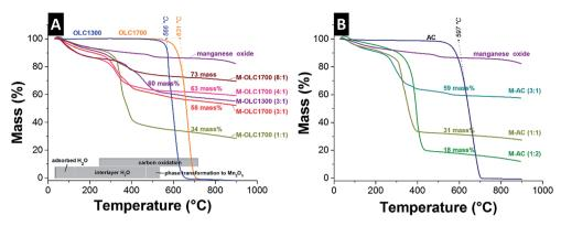
Fig. 3 TGA of the manganese oxide, the carbon powders, and the carbon/manganese oxide composites in synthetic air. All measurements were performed in synthetic air with a heating rate of 5 °C min<sup>-1</sup> for the carbon powders and 20 °C min<sup>-1</sup> for the hybrids. (A) Carbon onions and carbon onion/manganese oxide hybrids and (B) AC and AC/manganese oxide hybrids.
