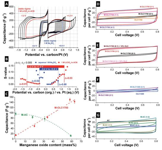
Fig. 6 (A) Potential window opening in a half-cell using M-OLC1700 (3:1) as working electrode, 1 mV s<sup>-1</sup> as scan rate and aqueous 1 M Na<sub>2</sub>SO<sub>4</sub> and 1 M LiClO<sub>4</sub> in ACN as electrolytes. (B) Corresponding S-values after Weingarth et al. (ref. 114). (C) Half-cell capacitance dependent on the manganese oxide loading. (D-G) Full-cell cyclic voltammograms at 10 mV s<sup>-1</sup> in aqueous 1 M Na<sub>2</sub>SO<sub>4</sub>.
