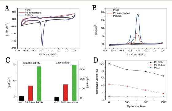
Fig. 10 Cyclic voltammograms of the PdCNs, Pd nanocubes, and commercial Pd/C, which are recorded at room temperature with a scan rate of  $50 \text{ mV s}^{-1}$  in (A) 1 M KOH solution; (B) 1 M KOH containing 1 M CH<sub>3</sub>OH; (C) the mass and specific activities (-0.2 V vs. SCE); (D) normalized current of 1500 cycles. Figure adapted from ref. 74 with permission.
