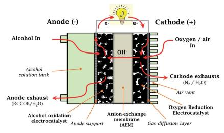
Fig. 1 Schematic of anion-exchange membrane-based direct alcohol fuel cell (AEM-DAFC).
