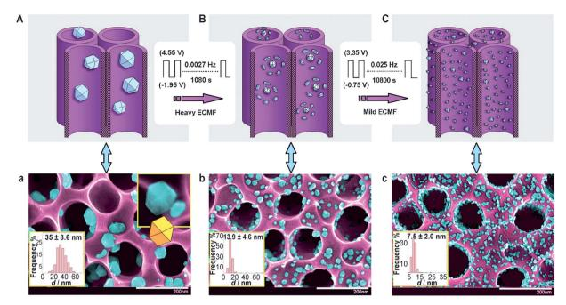
Fig. 11 (A) TNTAs with as-deposited Pd and (a) the corresponding SEM image. (B) TNTAs with Pd after heavy ECMF and (b) the corresponding SEM image. (C) TNTAs with Pd after heavy and mild ECFM and (c) the corresponding SEM image. False coloring of the SEM images shows Pd NPs (light blue) and the TNTA support (violet). The white scale bars in (a-c) are 200 nm. Figure adapted from ref. 82 with permission.
