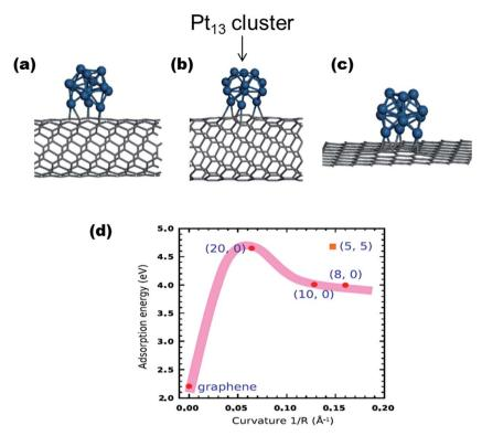
Fig. 3 The geometric structures of Pt<sub>13</sub> clusters adsorbed on carbon supports: (a) metallic (5, 5) SWNT, (b) semiconducting (10, 0) SWNT, and (c)  $(8 \times 8)$  graphene surface. (d) describes the dependence of the curvature of the carbon supports on the adsorption energy of Pt<sub>13</sub> clusters on the SWNTs and graphene sheet. Figure adapted from ref. 44 with permission.
