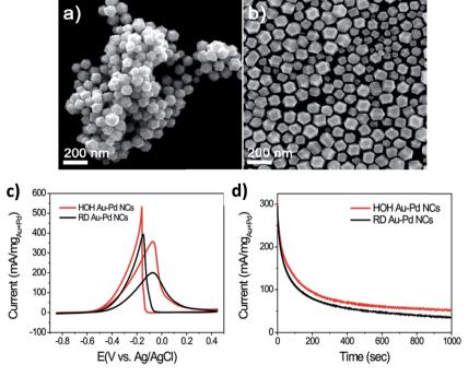
Fig. 9 SEM images of (a) HOH and (b) RD Au-Pd alloy NCs, (c) cyclic voltammograms of GCE-modified HOH and RD Au-Pd alloy NCs obtained in 0.1 M KOH + 0.5 M ethanol at a scan rate of 50 mV s<sup>-1</sup>, and (d) chronoamperograms of HOH and RD Au-Pd alloy NCs at -0.1 V vs. Ag/AgCl. Figure adapted from ref. 61 with permission.
