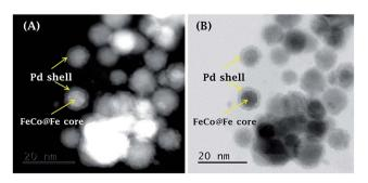
Fig. 7 (A) High-angle annular dark-field (HAADF)- and (B) bright-field (BF)-STEM images simultaneously acquired for FeCo@Fe@Pd/MWCNT-COOH. Figure adapted and modified from ref. 25 with permission.
