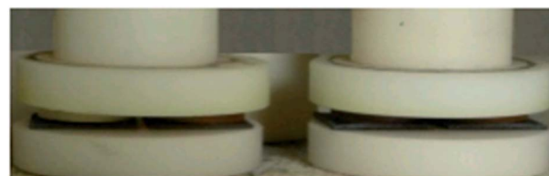
Fig. 1 Samples of CROFER 22 APU in contact with apatite pellets. Sets are kept under constant uniaxial pressure using alumina plates.
