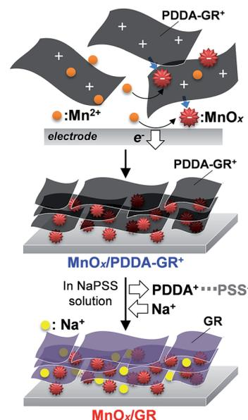
Scheme 1 Schematic of the synthesis of MnO<sub>x</sub>/GR film.
