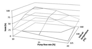
Fig. 4 Powder recovery as a function of inlet air temperature and pump flow rate for the sodium salt of 2-D-gluco-thiazolidine-4carboxylic acid
