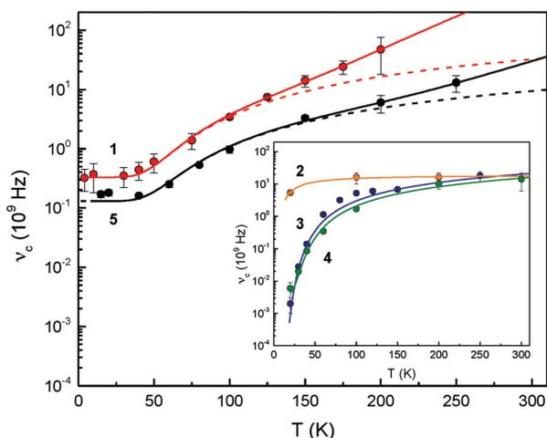
**Fig. 6** Temperature-dependent relaxation rates  $\nu_c = \tau_c^{-1}$  for complexes 1–5. The broken lines consider only the spin–spin and Orbach relaxation term of eqn (1) to illustrate the different contributions from Orbach and Raman type spin–lattice relaxation mechanisms. The full line represents the result of a least-squares fitting routine based on eqn (1).
