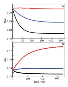
Fig. 3 Kinetics measured at 470 nm for B-TMF (5  $\mu$ M) at pH 4.6. A: after addition of B-TMF to an aqueous solution without added CB[7] (black) or addition to aqueous solutions of B-TMF containing 12 (blue) or 120  $\mu$ M CB[7] (red). B: after addition of water (black), or 12 (blue) or 470  $\mu$ M CB[7] (red) to B-TMF pre-incubated for 12 h at pH 4.6.
