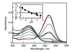
Fig. 1 Absorption spectra for B-TMF (18 µM) in water at different pH values after a 24 h equilibration period. The pH value for the highest absorbance for the band centered at 470 nm was 0.98 followed by pH values of 1.32, 1.80, 2.50, 3.01, 3.44, 3.86, 4.01, 4.61, 4.99, 5.45 and 6.04. Inset: Dependence of log  $(x_{Fl}/(1-x_{Fl}))$  with pH for solutions equilibrated for 2 h (black) and 24 h (red). The solid lines correspond to the fit of the data to eqn (\$12) in the ESI.†
