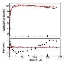
Fig. 5 Top: Fit of the binding isotherm for B-TMF ( $0.2~\mu M$ ) with CB[7] assuming a p $K_{ap}$  of 3.0 to a 1:1 stoichiometry (black, dashed line) and to sequential 1:1 and 1:2 B-TMF:CB[7] stoichiometries (red, solid line). Bottom: Residuals between the data and calculated values for the fits assuming a 1:1 stoichiometry (black) and sequential 1:1 and 1:2 stoichiometries (red).
