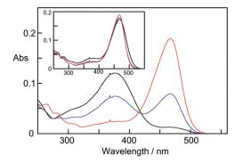
Fig. 2 Absorption spectra at pH 4.3 measured 7 h after the addition of B-TMF (5  $\mu$ M) in the absence (black) and presence of 12  $\mu$ M (blue) and 120  $\mu$ M (red) CB[7]. The inset shows the spectra right after the addition of B-TMF. For 120  $\mu$ M CB[7], the spectra are still unchanged 7 h after the addition of B-TMF.
