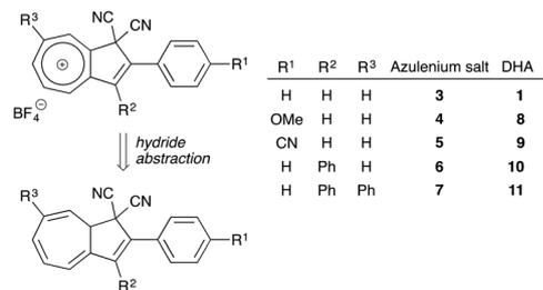
Fig. 1 Retrosynthetic route to azulenum salts 3–7 by hydride abstraction from DHA precursors 1, 8–11.
