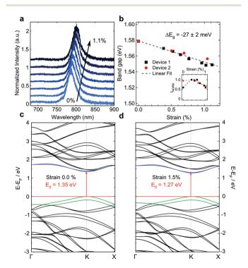
Fig. 3 (a) PL spectra for a single-layer MoSe<sub>2</sub> flake for increasing strains up to 1.1%. (b) Change in band gap for two single-layer samples (device 1 is from the spectra in (a)). The inset shows the normalized PL peak intensity for device 1 (black squares) and device 2 (red circles). (c) Calculated band structure of single-layer MoSe<sub>2</sub> including spin-orbit coupling at 0% strain and (d) at 1.5% uniaxial strain.
