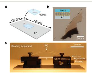
Fig. 1 (a) A viscoelastic (PDMS) stamp with exfoliated MoSe<sub>2</sub> is placed upside down onto a polycarbonate (PC) substrate to create a PC-MoSe<sub>2</sub>-PDMS stack. (b) Optical transmission image of a MoSe<sub>2</sub> flake sandwiched between PC and PDMS. The inset shows a cartoon of the sandwich for a single-layer flake. (c) Optical image of the apparatus used to bend the sandwich and apply strain to the MoSe<sub>2</sub> flake.
