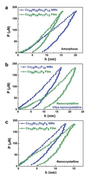
Fig. 4 Representative nanoindentation curves obtained from the films and individual nanowires, corresponding to: (a) the amorphous quaternary alloy, (b) the ternary nanocrystalline alloy and (c) the quaternary nanocrystalline alloy.
