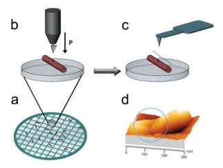
**Fig. 2** Schematic pictures of the indentation procedure, showing (a) an ensemble of NWs deposited dropwise onto the surface of an adherent coating previously deposited onto a TEM grid (which contained reference marks, not drawn), (b) the nanoindentation of a single NW using a conventional indenter tip, (c) subsequent imaging using an atomic force microscope (AFM) and (d) a real 3D AFM image corresponding to an indent performed onto a  $Co_{44}Ni_{30}Re_{12}P_{14}$  amorphous NW.
