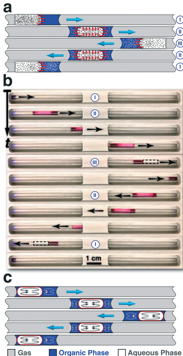
Fig. 3 (a) Microscale mixing of two immiscible fluids using oscillatory multiphase flow strategy for in situ studies of intra-phase transport processes. (b) Snapshot time-series of the oscillatory motion of a bi-phasic slug (clear phase: DI water, 15 μL, red phase: 1-octanol labelled with Sudan red, 10 μL, gas: pressurized nitrogen) in a tubular FEP reactor, during one complete oscillation cycle. (c) Ideal microscale mixing of two immiscible fluids using oscillatory multiphase flow strategy for in-flow studies of bi-phasic interfacial catalytic reactions. The available interfacial area for the multiphase process is highlighted in red. Adopted with permission from the American Chemical Society, 2015 (b). 69
