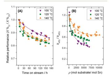
Fig. 8 (A) Relative catalytic activity of 10Sn-β over 170 h on stream between 100 and 140 °C. (B) Relative effective rate constant of 10Sn-β with respect to reactor turnover  $(\rho)$  and temperature.
