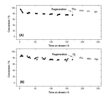
Time on stream data for 10Sn-β at 120 °C (A) and 140 °C (B).
