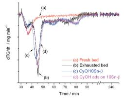
Fig. 6 TGA data for 10Sn- $\beta$ . The sample removed after  $\pm 500$  h on stream (b) is compared to a fresh catalyst sample (a), and two reference materials of 10Sn- $\beta$  doped with CyO (c) and CyOH (d).
