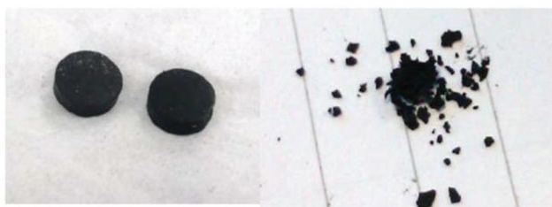
Fig. 8 Photograph of SBR 8 mm diameter disc samples before and after breakdown with G2 catalyst at room temperature over 24 h.
