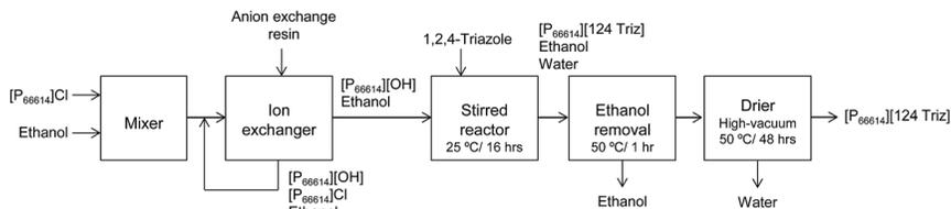
Fig. 2 Synthesis of  $[P_{66614}][124Triz]$  (adapted from Taylor *et al.*<sup>7</sup>).
