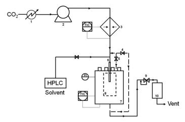
Fig. 1 Technical diagram of the Separex SAS equipment. (1) Chiller; (2) liquid pump; (3) heat exchanger; (4) and (5) by-pass valves, (6) co-axial nozzle for  $CO_2$  and metal salt solution delivery; (7) precipitation vessel; (8) sample recovery vessel; (9) back pressure regulator and (10) separation vessel.
