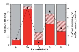
Fig. 10 Selectivity profiles of the AuPt/LaBO $_3$  catalysts compared to reported oxygen adsorption values for the relevant perovskite phases. Sum of the C $_3$  oxidation products (glyceric and tartronic acid) shown in solid red. C–C scission products (sum of glycolic acid, oxalic acid, formic acid and CO $_2$ ) shown in dashed red. Lactic acid selectivity shown by the solid grey bar. (In ) read from the second y axis represents the reported oxygen adsorption of the perovskite.
