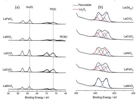
Fig. 8 XPS analysis of the  $AuPt/LaBO_3$  catalysts. (a) Au (4f) and Pt (4f) spectra of the catalysts. (b) La  $(3d_{5/2})$  spectra.
