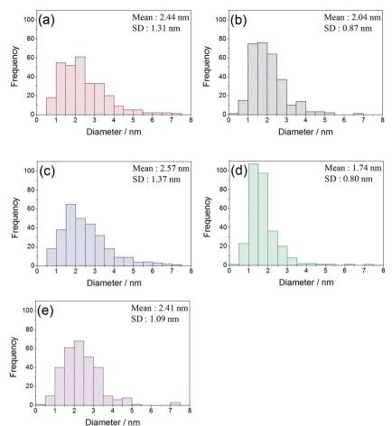
Fig. 5 Particle size distribution histograms of AuPt supported on the different SAS prepared LaBO $_3$  perovskites. (a) AuPt/LaCrO $_3$ ; (b) AuPt/LaMnO $_3$ ; (c) AuPt/LaFeO $_3$ ; (d) AuPt/LaCoO $_3$ ; (e) AuPt/LaNiO $_3$ .
