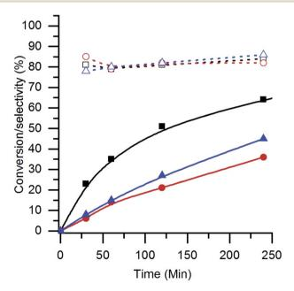
Fig. 13 Conversion and  $C_3$  oxidation product selectivity of  $AuPt/LaMnO_3$  using different perovskite preparation routes. Conversions are represented with solid fills ( $\blacksquare = SAS$ ,  $\blacktriangle = flame$  pyrolysis and  $\bullet = mechanochemical$ ) and selectivities with the corresponding open symbols.
