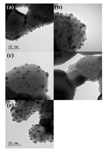
Fig. 4 Representative transmission electron micrographs of AuPt supported on the different SAS prepared LaBO $_3$  perovskites. (a) AuPt/LaCrO $_3$ ; (b) AuPt/LaMnO $_3$ ; (c) AuPt/LaFeO $_3$ ; (d) AuPt/LaCoO $_3$ ; (e) AuPt/LaNiO $_3$ .
