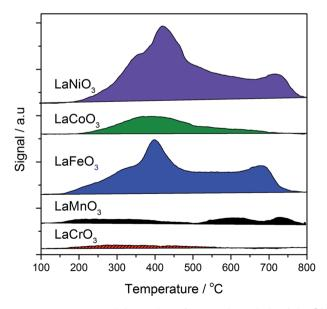
Fig. 9 Temperature programmed desorption of ammonia analysis of the SAS prepared LaBO<sub>3</sub> supports, where B is: Cr (red solid); Mn (black); Fe (blue); Co (green); or Ni (purple).
