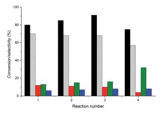
Fig. 12 Re-use testing of the AuPt/LaMnO<sub>3</sub> catalyst. Black fill = glycerol conversion; black dashed = glyceric acid selectivity, red fill = tartronic acid selectivity; green fill = C-Cscission selectivity and blue fill = lactic acid selectivity. Conditions: glycerol 0.3 M in water, 4 : 1 NaOH : glycerol, glycerol : metal = 1000, 3 bar  $O_2$ , temperature = 100 °C.
