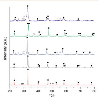
Fig. 3 Powder X-ray diffraction patterns of the SAS La: B precipitates after 750 °C calcination. In ascending order, the B site samples are: Cr (red); Mn (black); Fe (blue); Co (green); and Ni (purple). Phases:  $\bullet$  perovskite phases (for simplicity, the rhombohedral, orthorhombic and cubic phases are not differentiated);  $\bigcirc$  Fe<sub>2</sub>O<sub>3</sub>;  $\bigcirc$  La<sub>2</sub>O<sub>3</sub>;  $\square$  Co<sub>3</sub>O<sub>4</sub>; and X La<sub>2</sub>CrO<sub>6</sub>.
