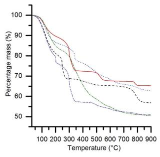
Fig. 2 Thermogravimetric analysis of the SAS precipitated materials, where the B site element is: Cr (red solid); Mn (dashed black); Fe (blue dotted); Co (green dashed-dotted); and Ni (purple dashed-dotted). The experimental conditions used were:  $10\,^{\circ}$ C min<sup>-1</sup> ramp rate, 50 ml min<sup>-1</sup> flow rate of air and 15–25 mg of sample.
