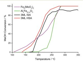
Fig. 7 Methanol conversion during the TPPFR over bulk and shell@core iron molybdate catalysts.
