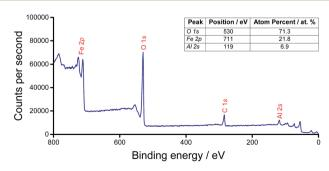
Fig. 1 Widescan XPS spectrum of  $Al_xFe_{(2-x)}O_3$  and table, inset, of the associated surface composition.
