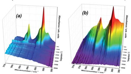
Fig. 6 3D maps of the C-H region of the IR spectra during TPD of methanol from the (a) 3ML@ISA and (b) 3ML@HSA catalysts.
