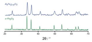
Fig. 2 XRD powder patterns of  $Al_x Fe_{(2-x)}O_3$  and a phase-pure haematite reference sample.
