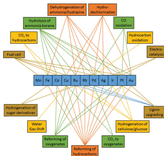
Fig. 8 Different guest metals in bimetallic NiM catalysts and their corresponding catalytic applications.
